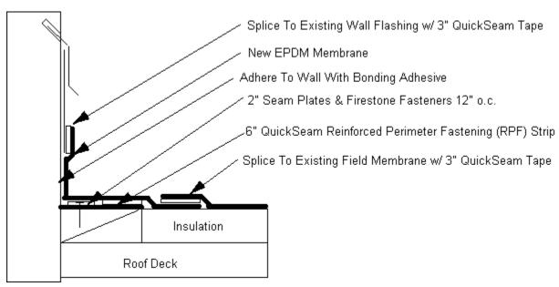
Note: The application of QuickSeam Tape to existing in-service EPDM membrane requires special cleaning and priming procedures. Refer to Section F - "Cleaning and Priming of In-Service EPDM Membrane.
